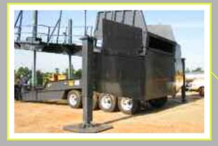
Outrigger Protector made of heavy square tubing to protect the rear outrigger cylinders. This prevents damage to the ram of the cylinder as material is pushed away from the rear of the tipper.
