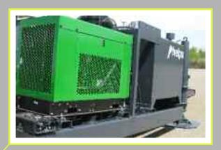
Hydraulic Power Unit complete with John Deere engine with enclosure, hydraulic reservoir, pumps, valves and filters. Mounted to passenger side of tipper frame.
