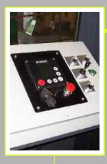
**Control Panel** that is simple to use and easy to maintain. Includes features such as engine auto-throttle and deck anti-jog.
